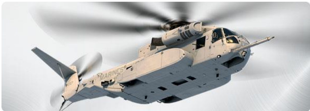
Sikorsky CH-53K powered by three General Electric T408-GE-400s
