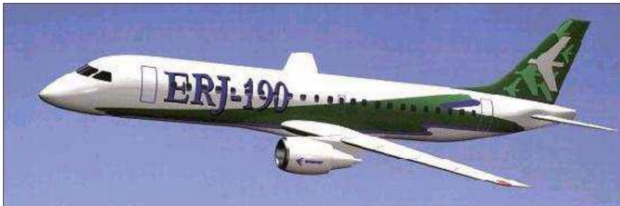
Embraer 190 powered by two CF34-10E5s
