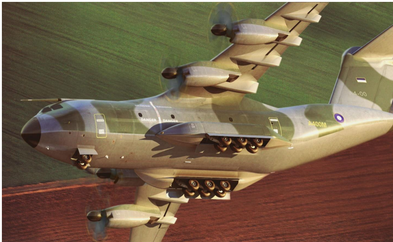
Airbus A400M powered by four TP400-D6s
