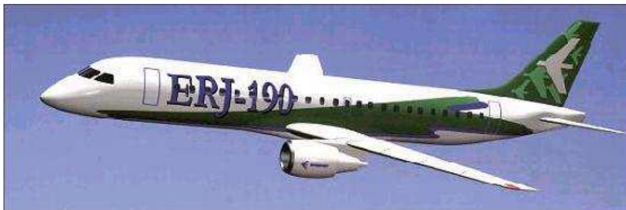
Embraer 190 powered by two CF34-10E5s
